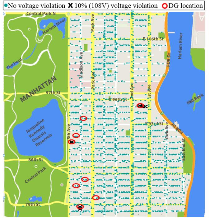
Fig. 4. Geographical voltage distribution in Yorkville network for 8% voltage reduction of the peak hour of the year. Eight voltage violations are detected exceeding 10% (under 108 V) out of 2282 structure points. Underlying map ©2014 by Google.
